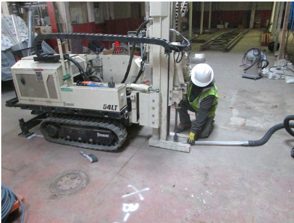
Photo 14: ECA staff drilling at Boring 1 inside the former garage structure
