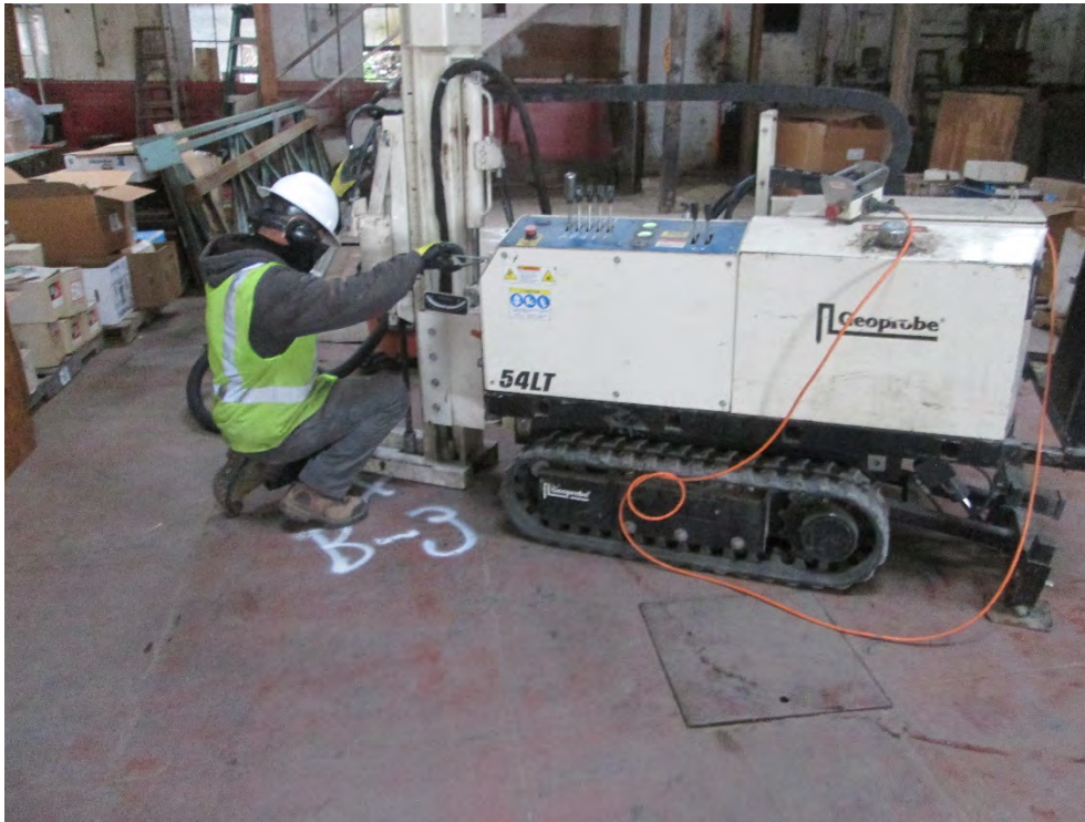
Photo 5: ECA staff drilling at Boring 3 nearby the inground hoist
