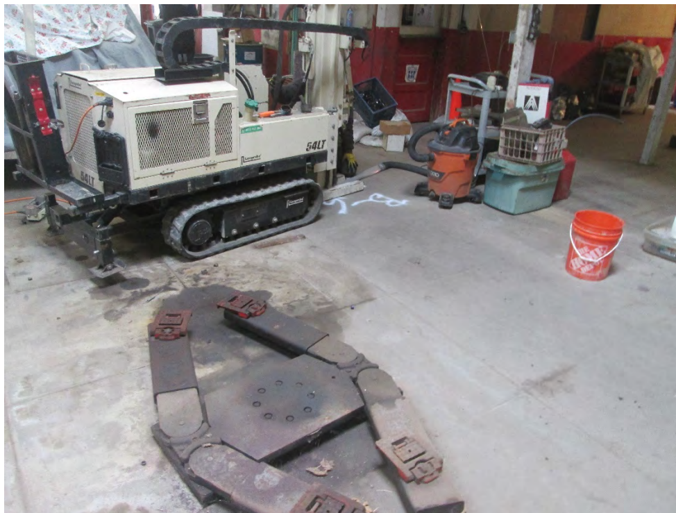
Photo 16: ECA staff drilling at Boring 6 neaby the inground hoist
