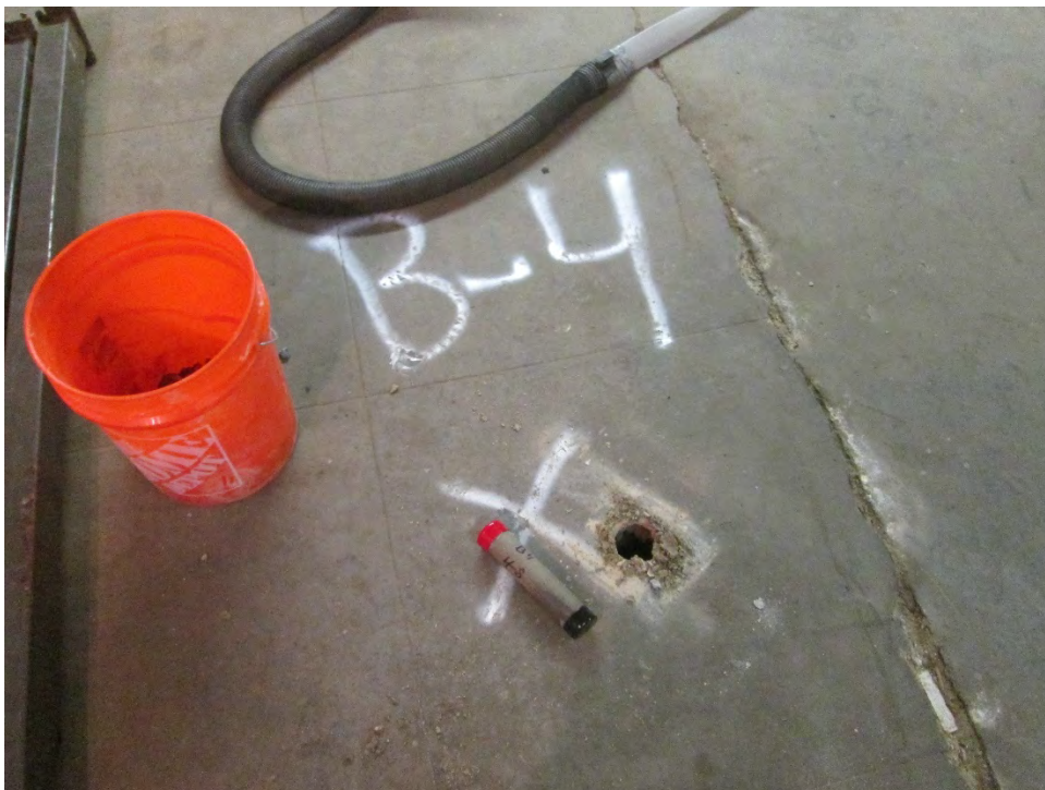
Photo 20: Soil sample at Boring 4 nearby the replaced concrete area
