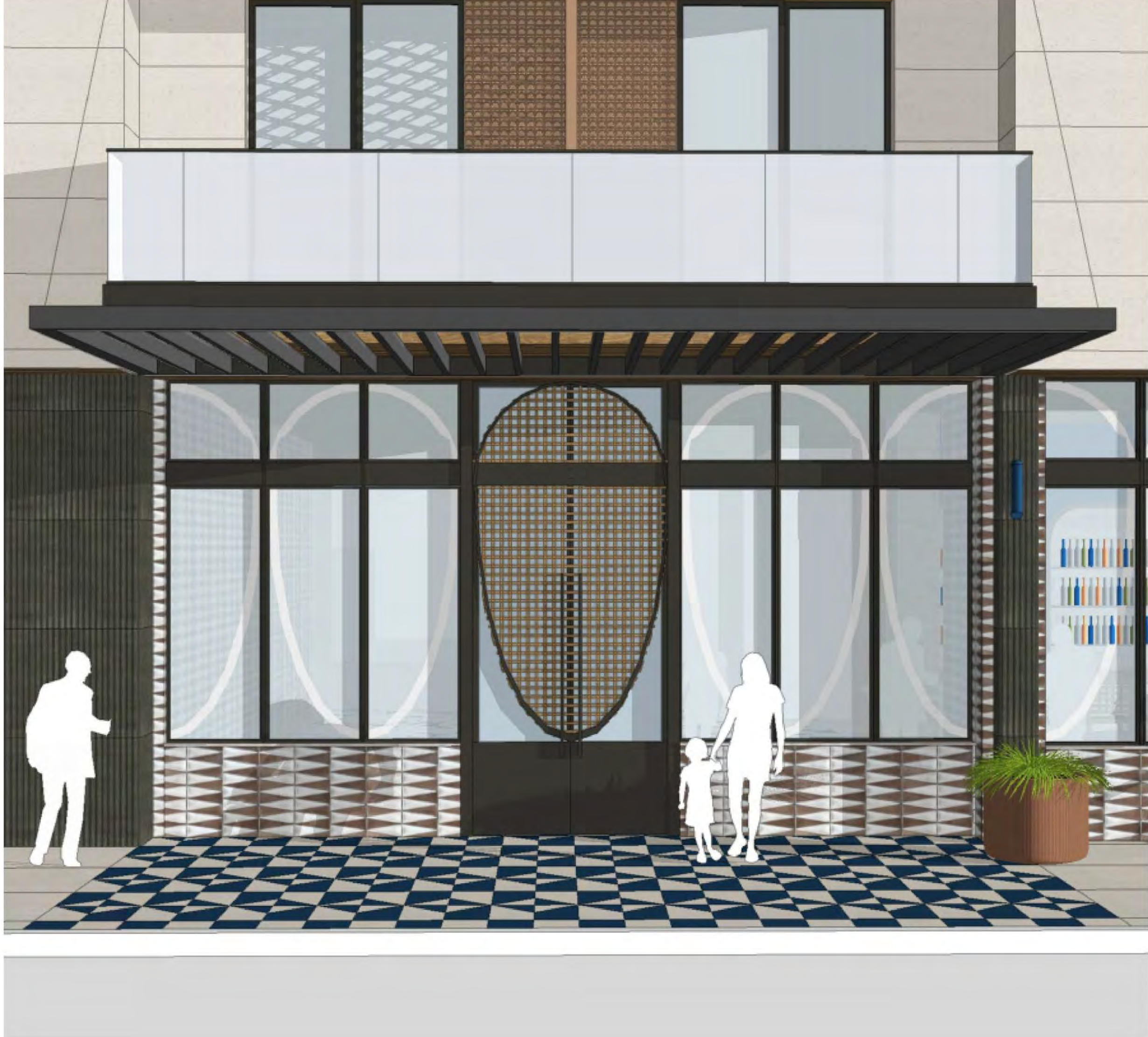
CLADDING - DECORATIVE TILE 01 - DIMENSIONAL CONCRETE TILE, DARK GRAY CLADDING - DECORATIVE TILE 02 - DIMENSIONAL ANGLED TRIANGLE TILE, TWO TONE CLADDING - PORCELANOSA MAKER SMOKE CLADDING - PORCELANOSA MAKER ROPE CLADDING - PORCELANOSA MANHATTAN COGNAC CUSTOM CUT METAL PANEL - BRONZE METAL - DARK BROZE BOARD FORMED CONCRETE COLUMNS
