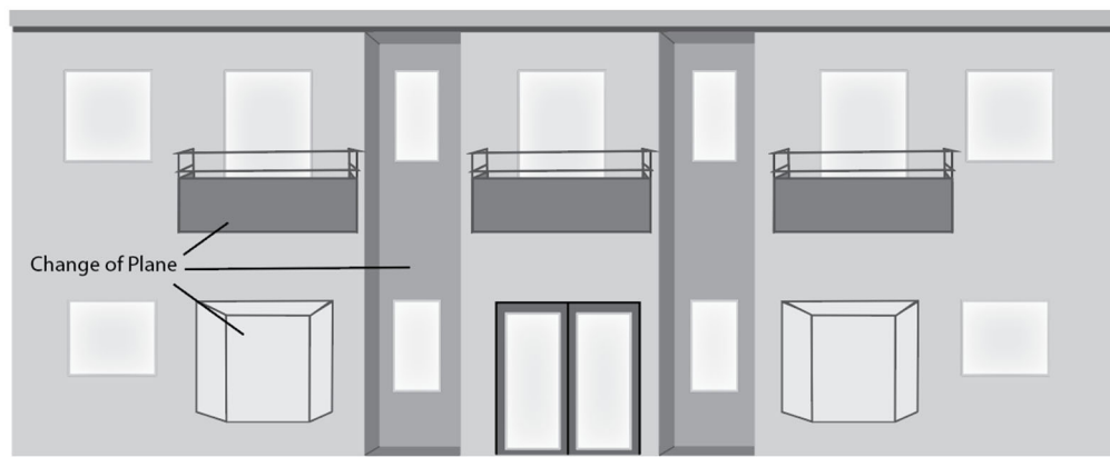
522 Figure 11: Change of Plane on Primary Façade
