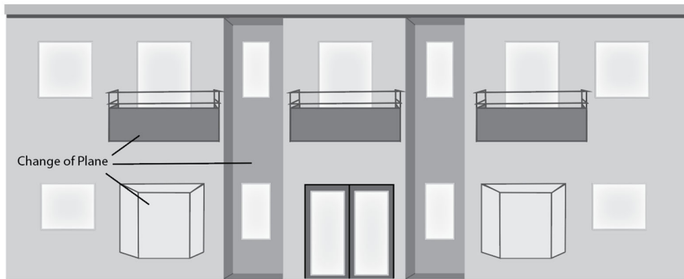
502 Figure 11: Change of Plane on Primary Façade
