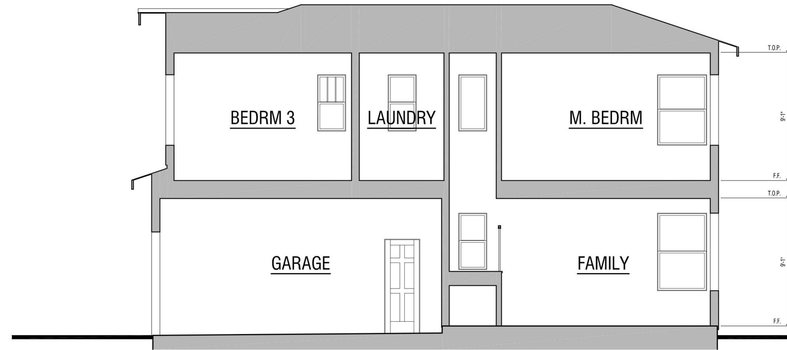
Building Section A-A
