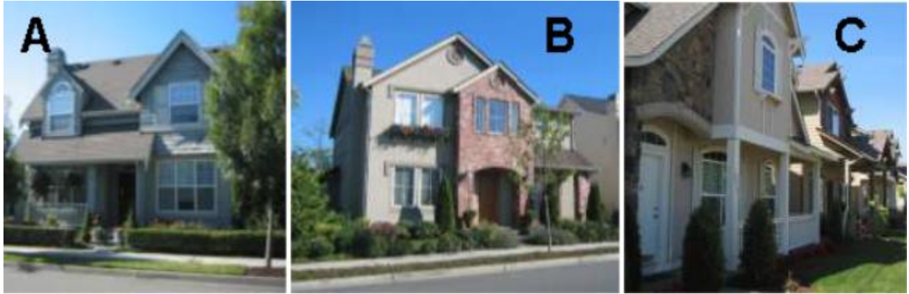
Figure 7. Examples of how houses can meet architectural detail criteria. Image A includes decorative windows, building material treatment, and roofline elements. Image B includes decorative brick use, window treatments, entry design, and ventilation circles. Image C includes decorative building materials, door/entry feature, windows, and roofline elements.
