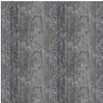
P5. BOARD FORMED CONCRETE
