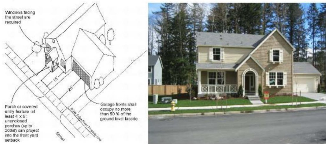
Figure 1: Garage placement/frontage standards and design.
