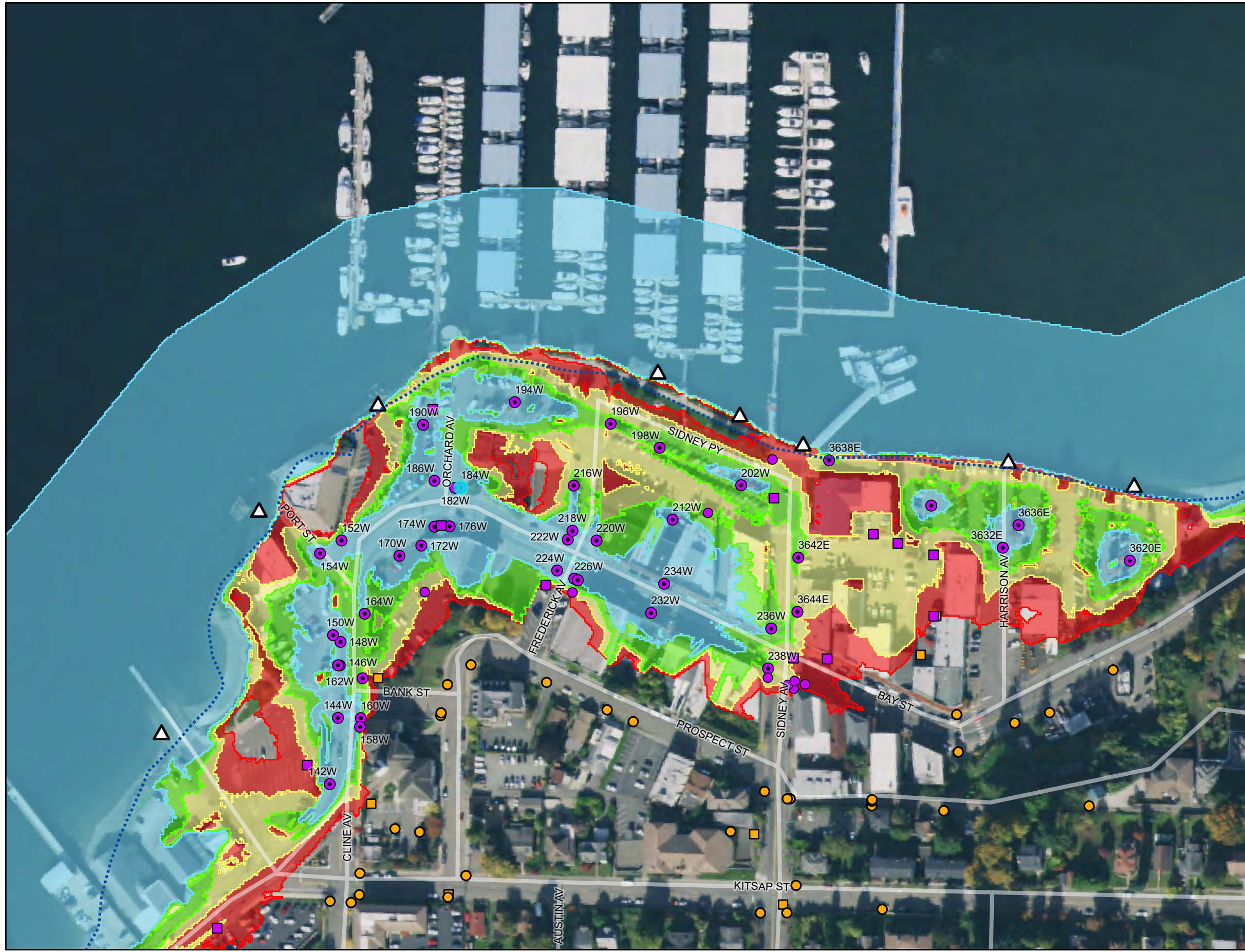
Figure 4. Projected 100 Year Marine Flood Extent Under Sea Level Rise Scenarios: Port Orchard Marina
