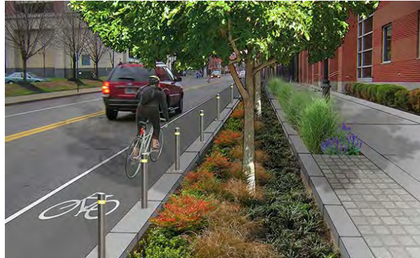
Figure 16: Low Impact Development Stormwater Management Techniques incorporated into street design. This sort of design is encouraged in the Ruby Creek neighborhood.
