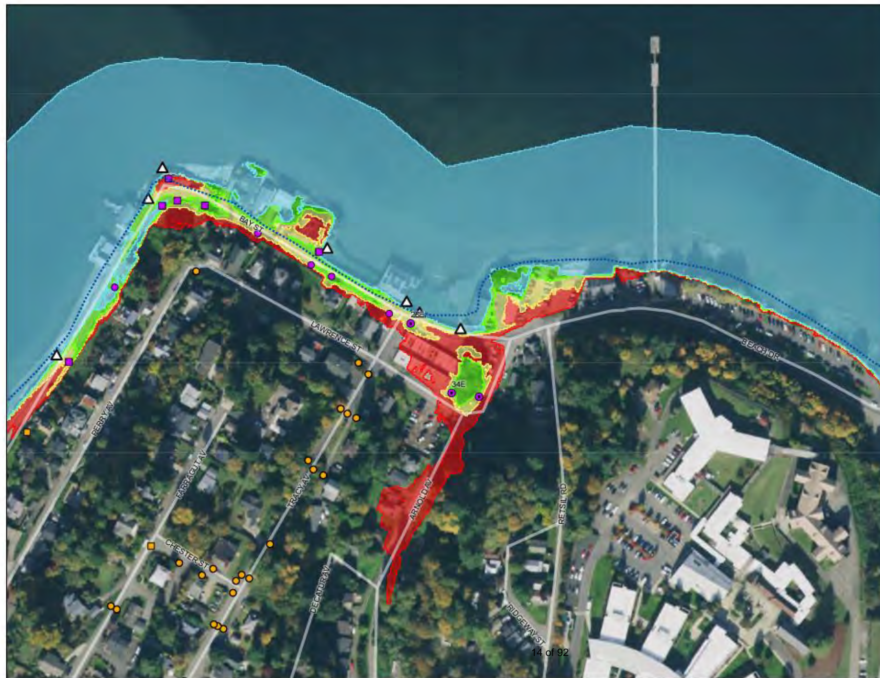
Figure 6. Projected 100 Year Marine Flood Extent Under Sea Level Rise Scenarios: Annapolis to Foot Ferry Terminal
