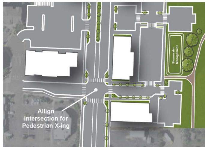
**Figure 20: Align driveways to facilitate pedestrian crossings throughout the Sidney Road SW corridor.**
