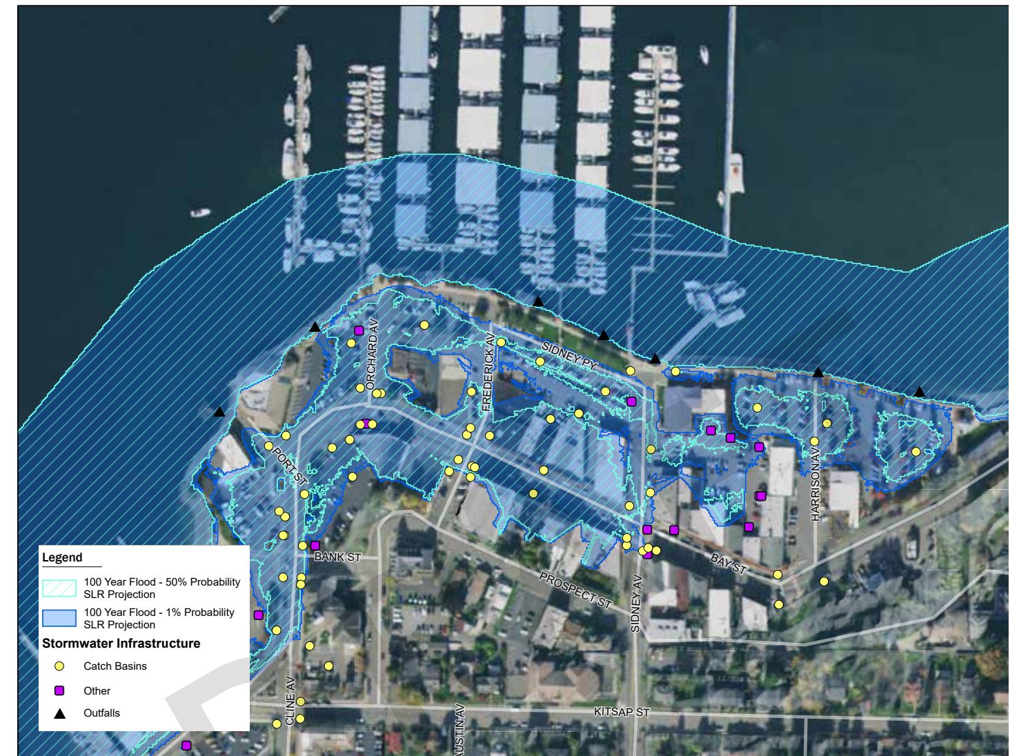
PROJECTED 100 YEAR FLOOD EXTENT UNDER SEA LEVEL RISE SCENARIOS: PORT ORCHARD MARINA
