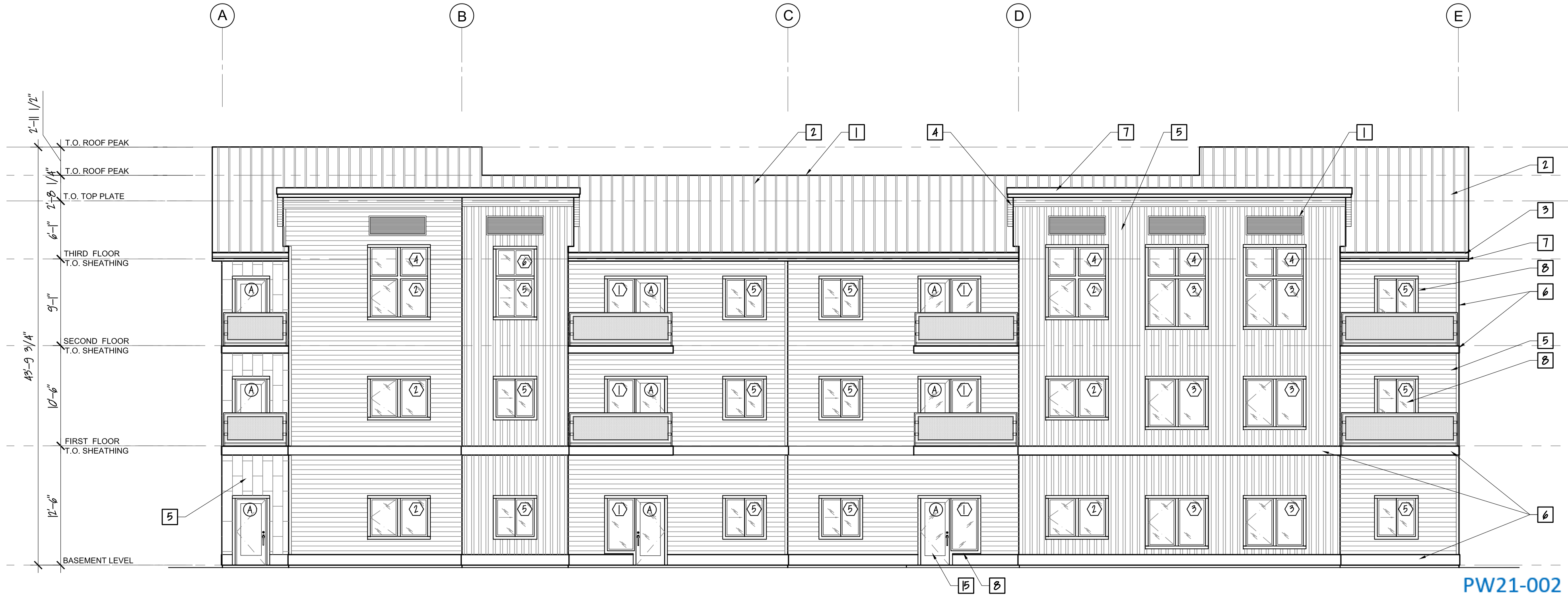
2 EXT. ELEVATION - SOUTH FACADE @ SOUTH BUILDING SCALE: 1/8"=1'-0"
