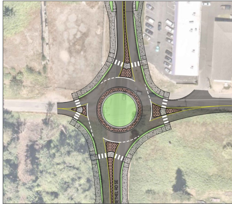
4-Leg Single Lane Roundabout Salmonberry/Bethel
