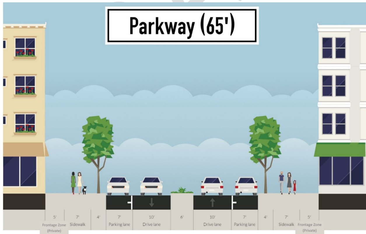
Parkway Example Cross-Section – 65' Right-of-Way Width
