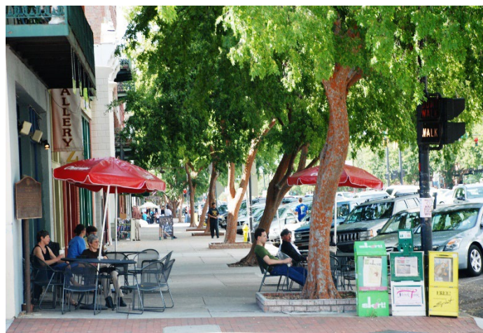
Sidewalk with frontage zone, pedestrian through zone, and street furnishing zone
