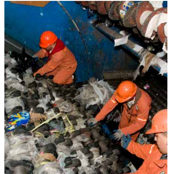
The sorting equipment is filled with plastic bags. Twice a day employees have to shut down the entire system so they can crawl onto the screen and use knives to cut away the plastic (Waste Connections)
