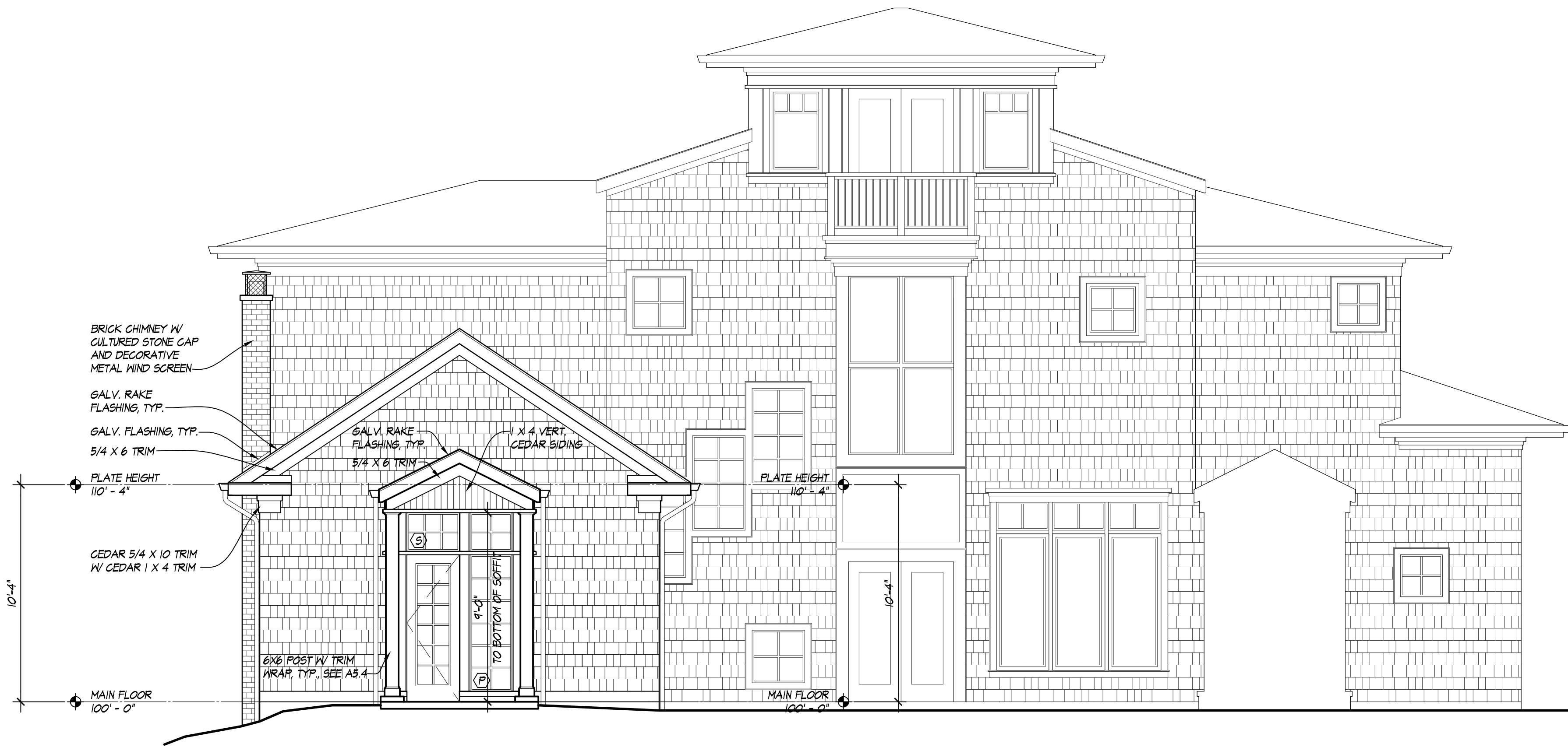
WEST ELEVATION: FAMILY ROOM 1/4" = 1'-0"
