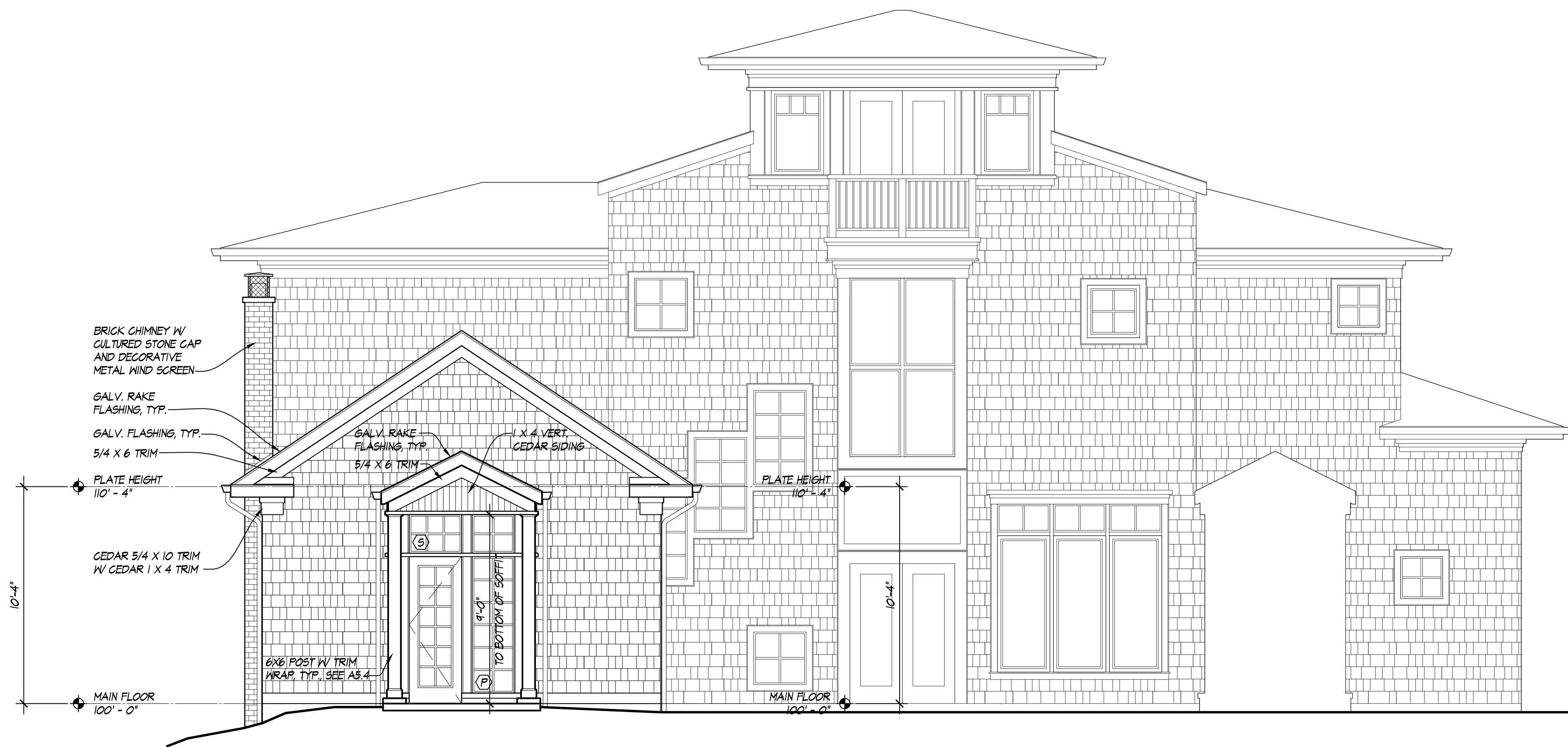
WEST ELEVATION: FAMILY ROOM 1/4" = 1'-0"
