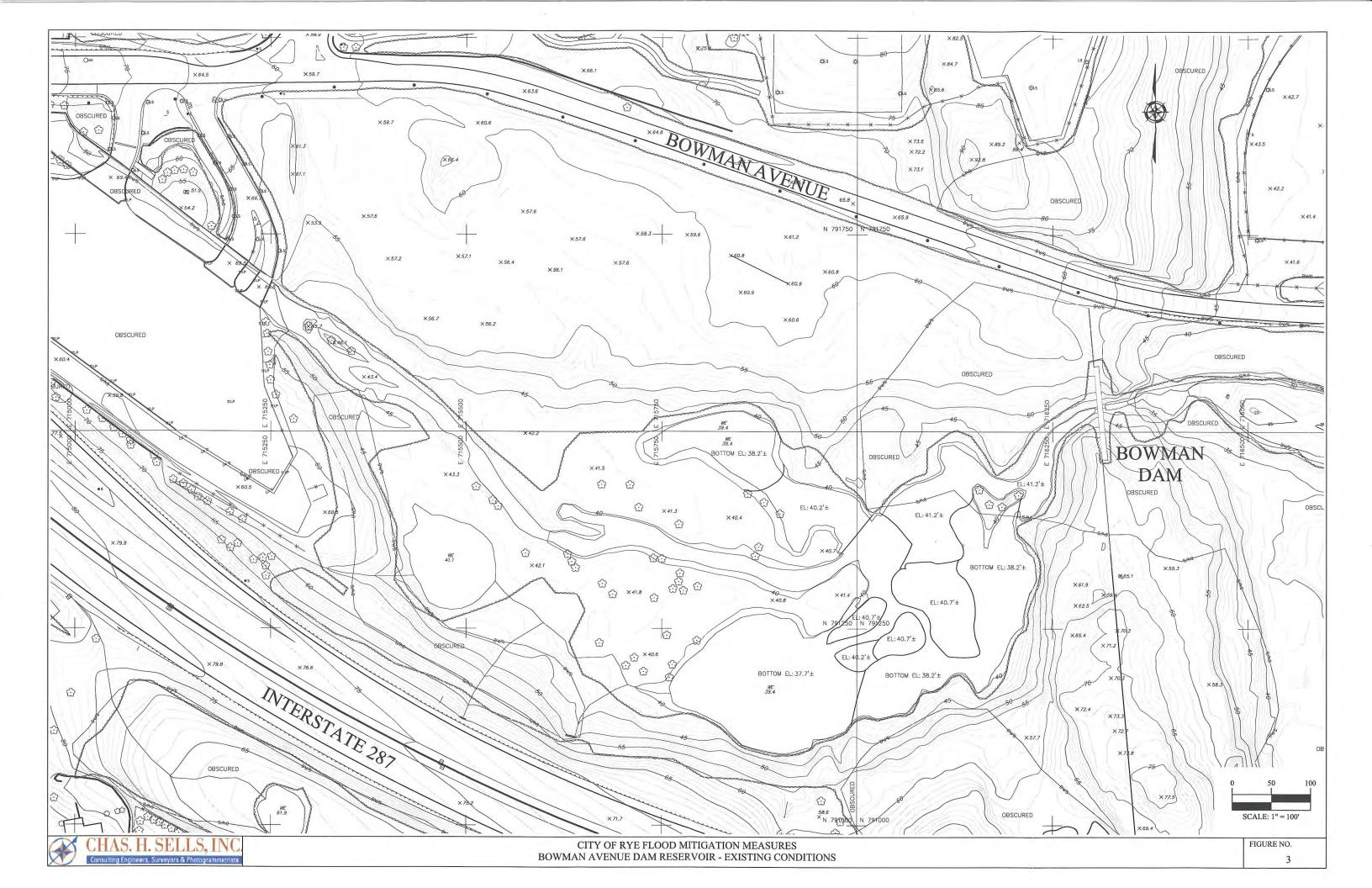
of the pond has been formed as a result of dumping within the last 25-years. The maximum depth of the pond is 30-feet as determined by soundings performed by Sells.
