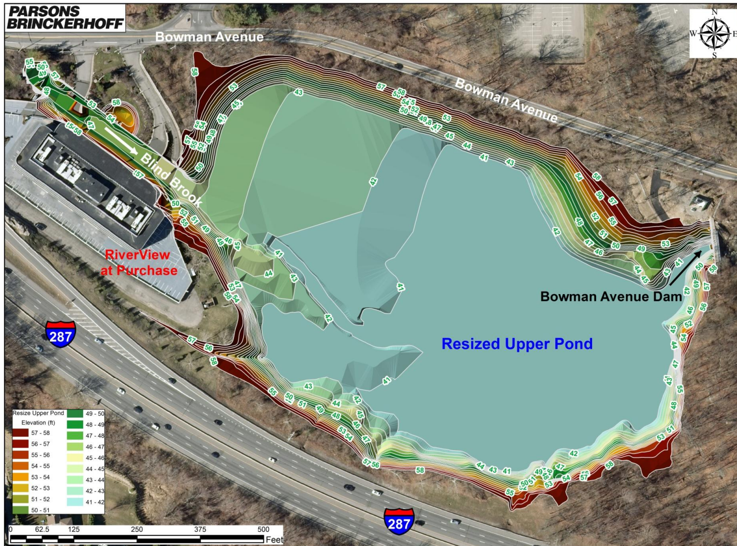
Figure 35 - Proposed TIN and 1-foot Interval Contours of Resize Upper Pond
