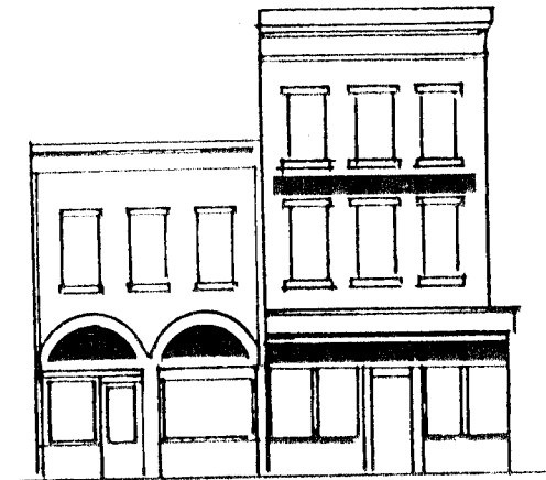
In many buildings, a logical place for a sign is built into the facade design. Examples of this "signable area" are shown here in block.
