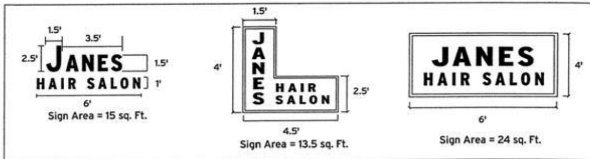
Figure 14.19-2 Measuring Surface Sign Area
