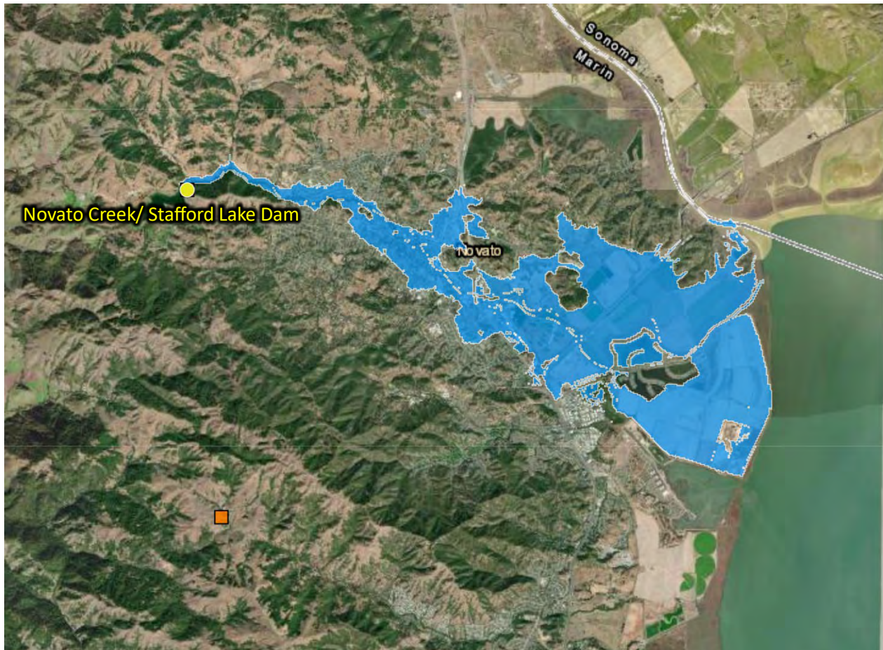
Figure 3.13: Novato Creek/ Stafford Lake Dam Inundation Area
