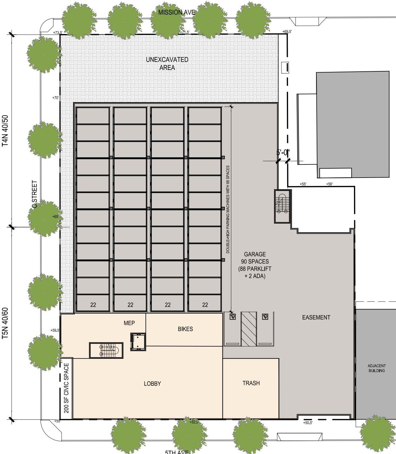
BASE PLAN AT GROUND LEVEL / BASEMENT
