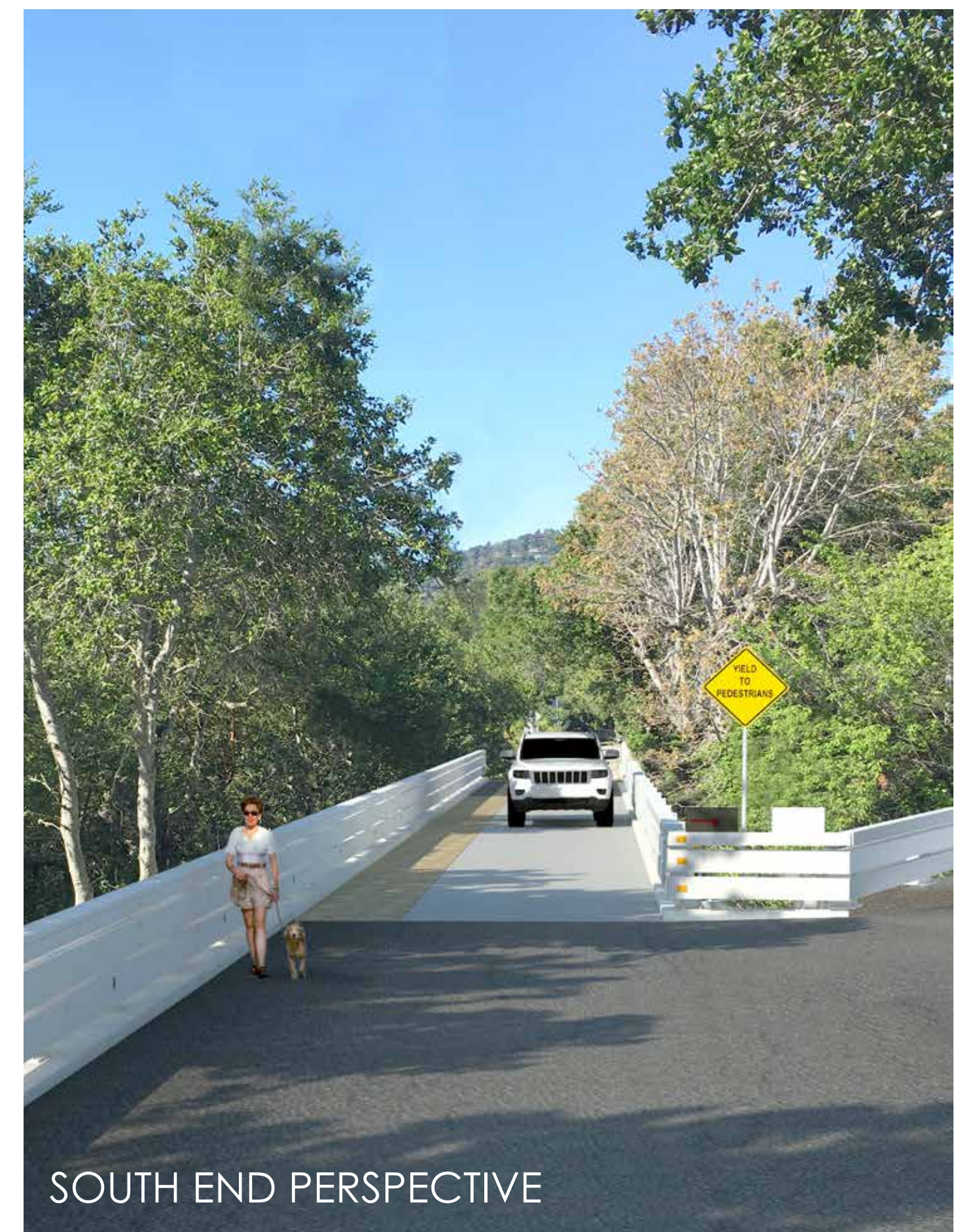
WOOD PLANK STAMPED & COLORED CONCRETE BRIDGE SURFACE
