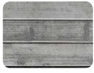
BOARD FORM CONCRETE
