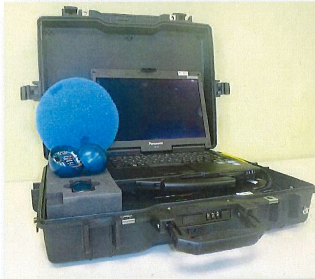
Figure 1: SmartBall Core, Foam Outer Shell, and SBR
