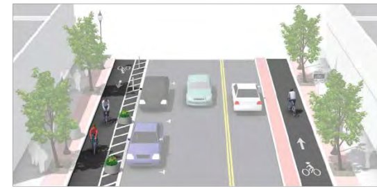
CLASS IV: SEPARATED BIKEWAYS A new class of bikeway that are typically on-street and physically separated from motor vehicle traffic by a vertical barrier such as a curb, on-street parking, bollards, planters, or stormwater infrastructure. They can provide one-way or two-way travel for bicyclists.
