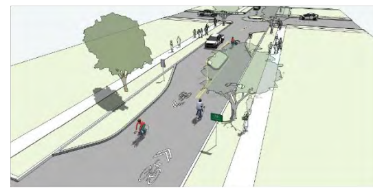
CLASS III+: BIKE BOULEVARD A Class III Bicycle Route can become a bicycle boulevard if paired with traffic calming infrastructure such as curb extensions, chicanes, and diverters.
