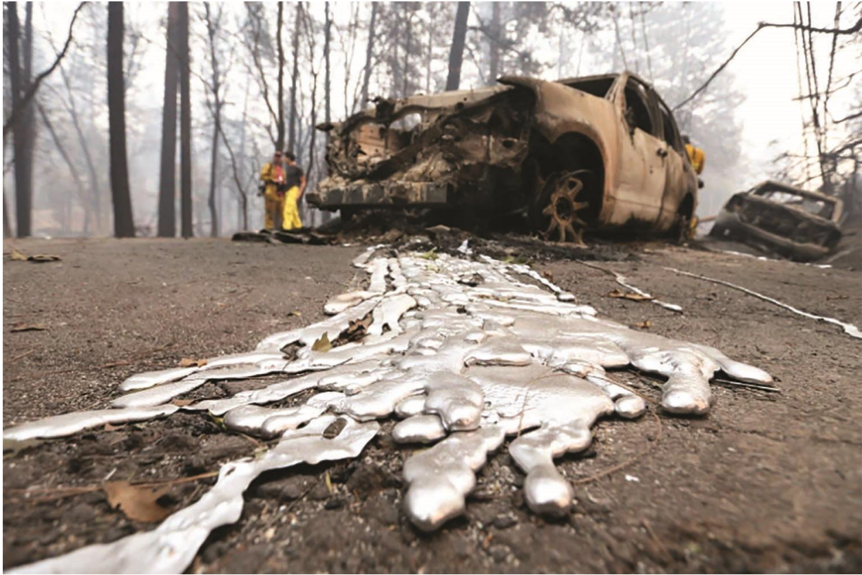
Burned Cars and Melted Aluminum from Engine Block Caused by Extreme Heat in Camp Fire, November 2018. (Jane Tyska/Bay Area News Group) The Mercury News . Published Nov. 13, 2018.
