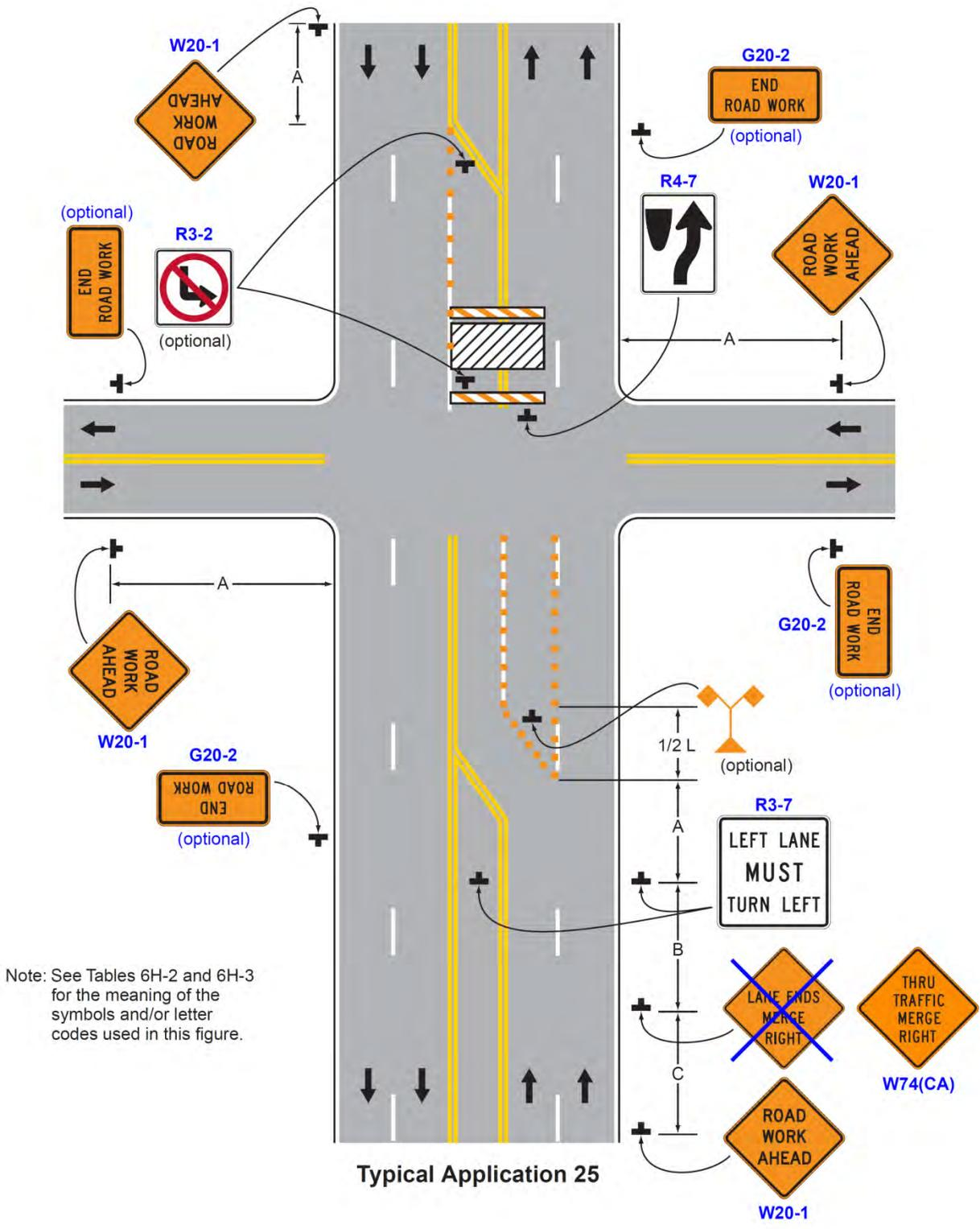
**Figure 6H-25A (CA). Multiple Lane Closures at an Intersection (TA-25A(CA))**
