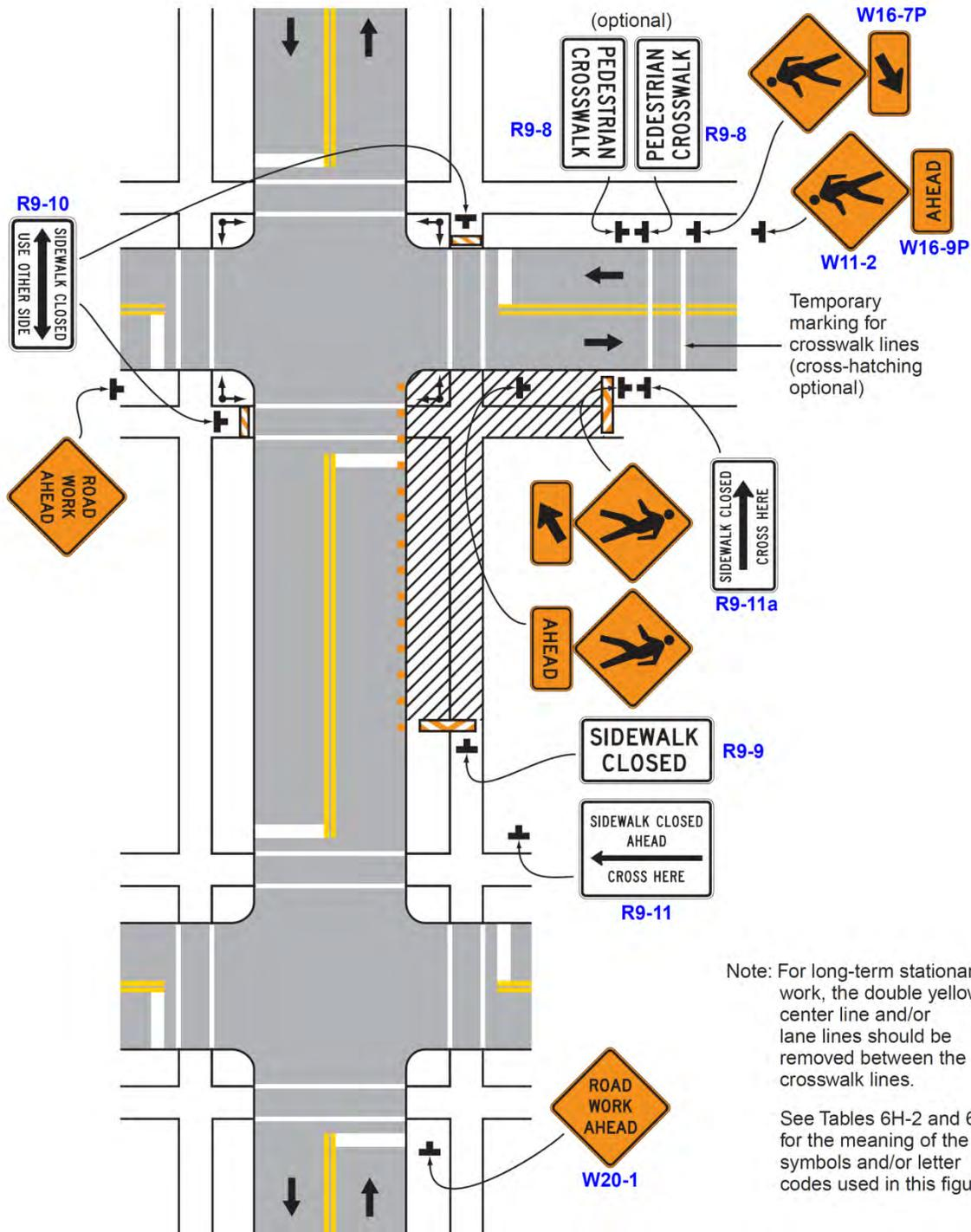
Note: For long-term stationary work, the double yellow center line and/or lane lines should be removed between the crosswalk lines.
