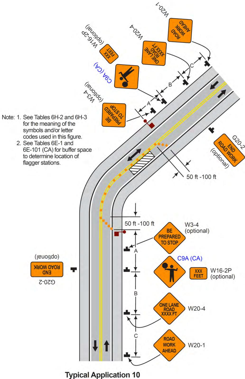
**Figure 6H-10A (CA). Lane Closure on Two-Lane Road Using Flaggers (TA-10A) Using Portable Transverse Rumble Strips**
