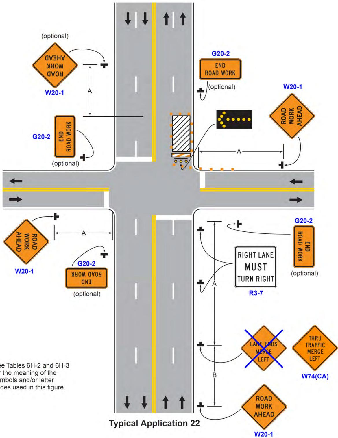
**Figure 6H-22A(CA). Right-Hand Lane Closure on the Far Side of an Intersection (TA-22A (CA))**
