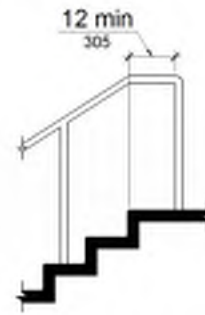
FIGURE 11B-505.10.2 TOP HANDRAIL EXTENSION AT STAIRS
