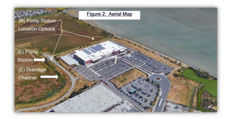
As indicated in the geotechnical report, the planned pump station is feasible from a geotechnical standpoint. The weight of the new pump station is anticipated to be less than the weight of the excavated soil to build the station.
