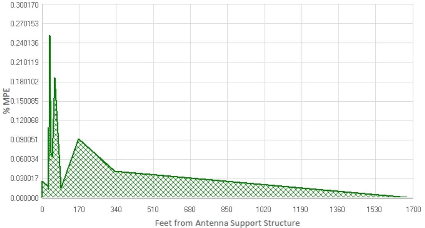
Maximum power density at ground level: 2.53  $\mu\text{W}/\text{cm}^2$
