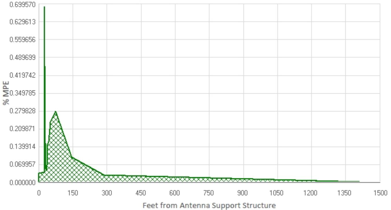
Maximum power density at ground level: 6.9  $\mu\text{W}/\text{cm}^2$
