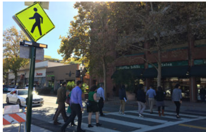
Figure 6.15 Examples of pedestrian strategies recommended for Downtown San Rafael: (right) a pedestrian crossing with a flashing beacon, and (far right) an enhanced mid-block pedestrian crossing with a high-visibility crosswalk.
