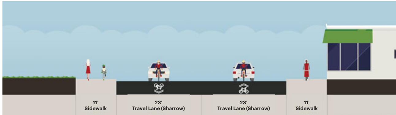
Existing condition (46' Curb-to-Curb)
