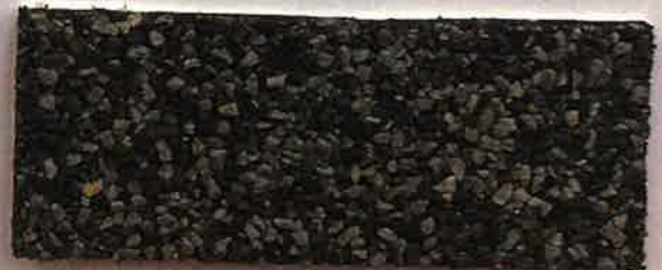
ASPHALT SHINGLES "COLONIAL SLATE" ROOFING, TYPICAL
