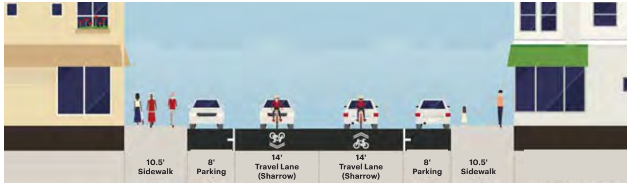
Existing condition (44' Curb-to-Curb)
