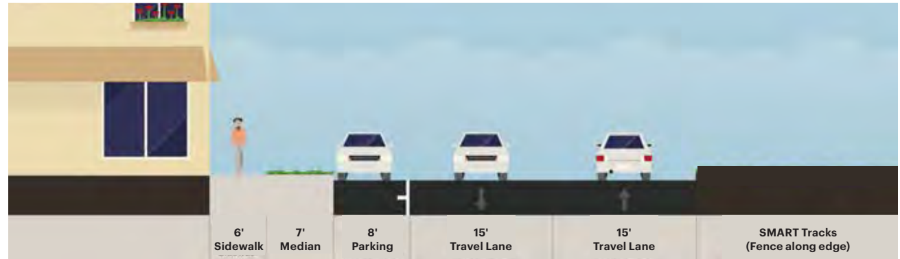
Existing condition (36' - 38' Curb-to-Curb)
