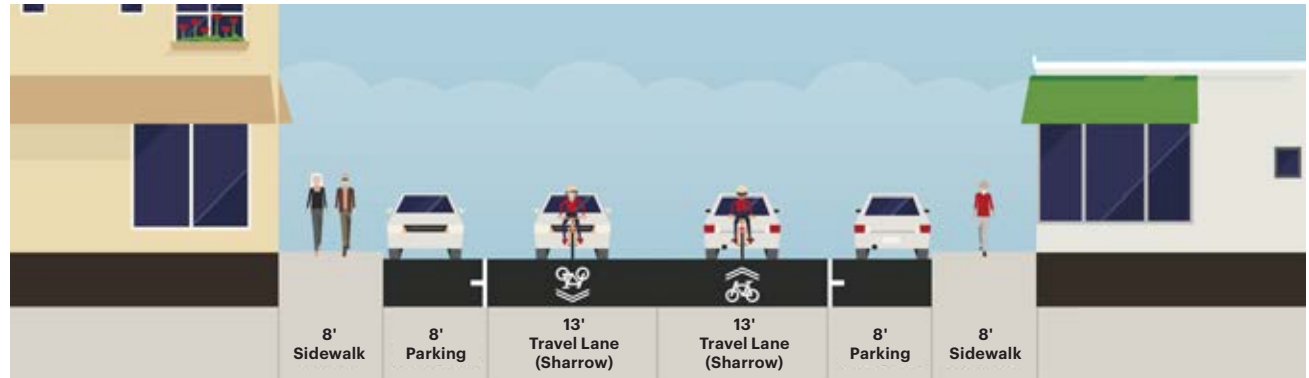
Existing condition (42' Curb-to-Curb)
