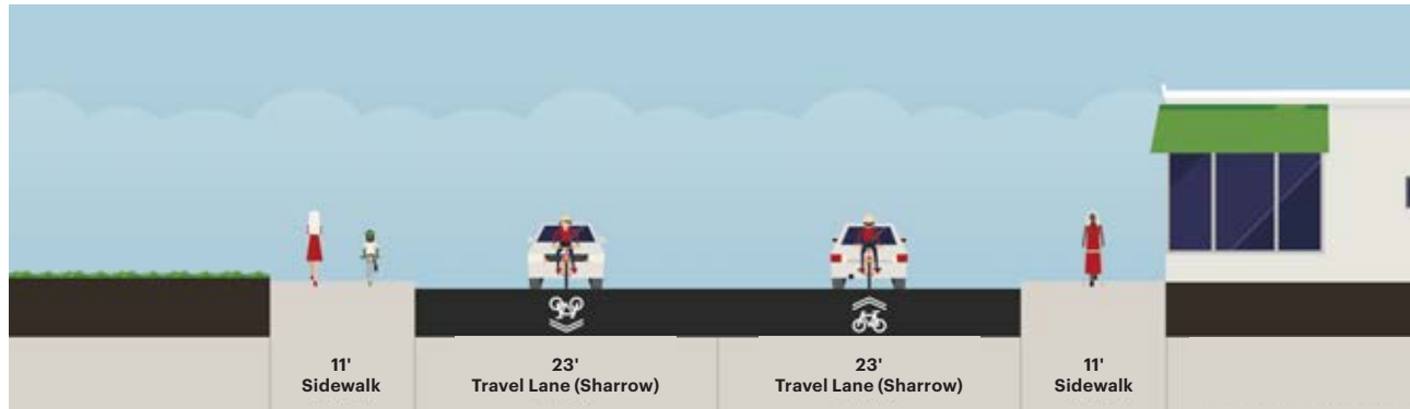
Existing condition (46' Curb-to-Curb)
