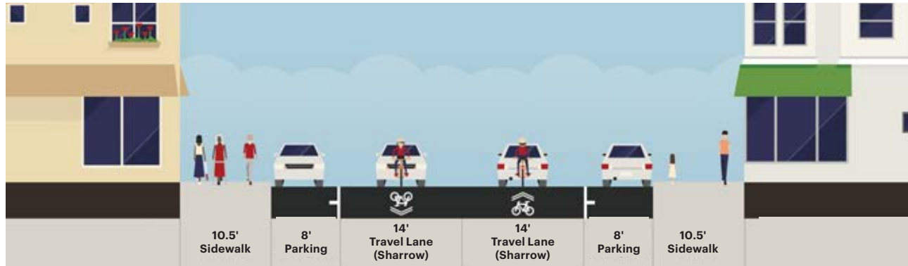
Existing condition (44' Curb-to-Curb)
