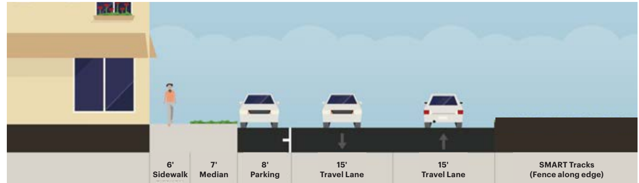
Existing condition (36' - 38' Curb-to-Curb)
