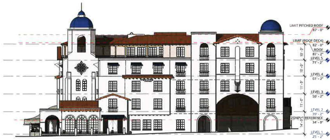
2 EAST ELEVATION - PROPOSED DRB DESIGN 1/16" = 1'-0"
