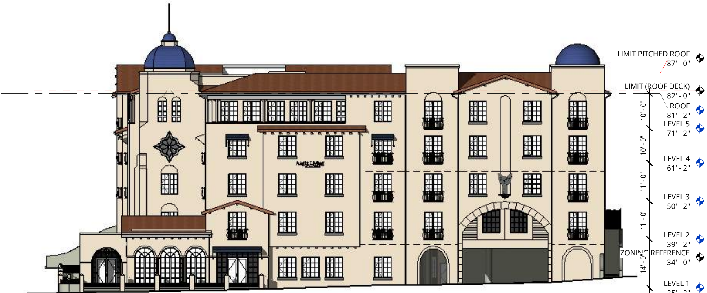
3 EAST ELEVATION - PROPOSED DRB DESIGN 1/16"=1'-0"
