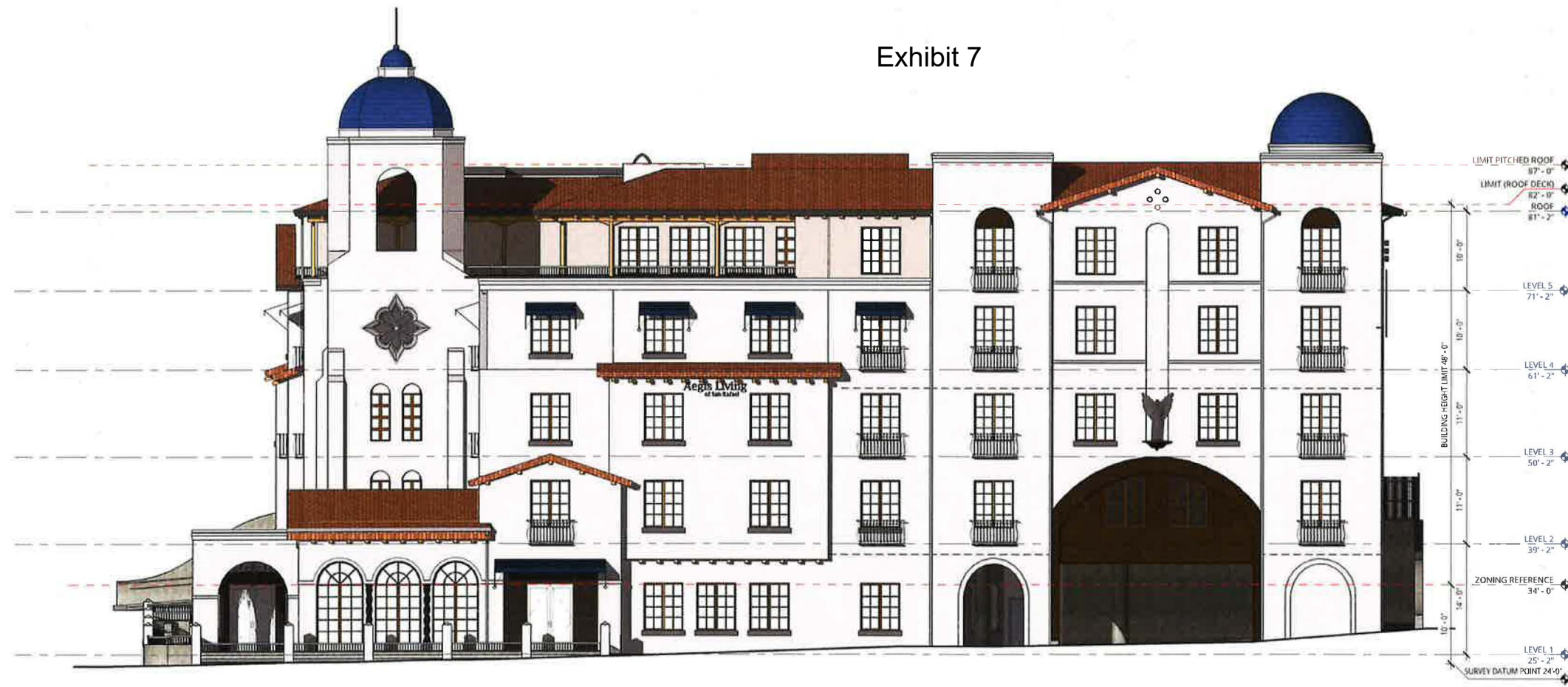
1 EAST ELEVATION - PROPOSED DESIGN 1/8" = 1'-0"
