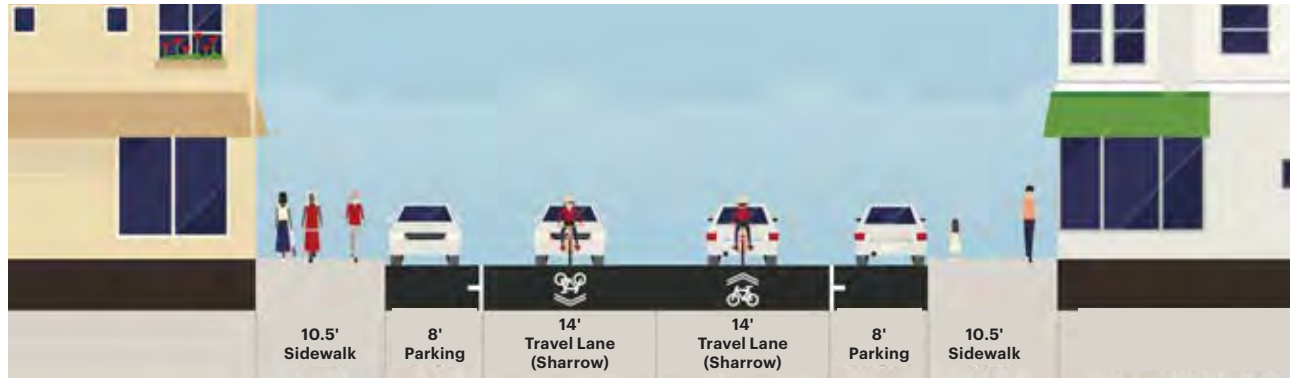
Existing condition (44' Curb-to-Curb)
