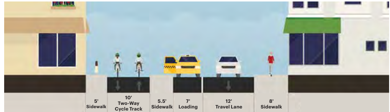
Near-term transformation (34.5' Curb-to-Curb)
