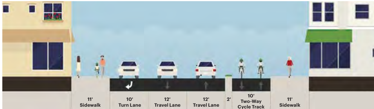
Near-term transformation (46' Curb-to-Curb)
