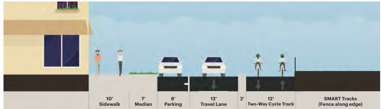
Near-term transformation (34' Curb-to-Curb)
