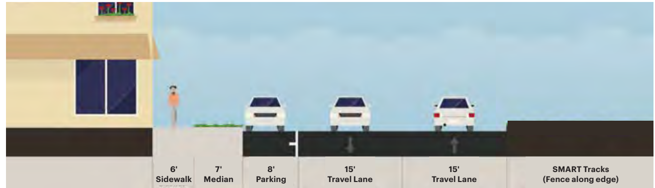
Existing condition (36' - 38' Curb-to-Curb)
