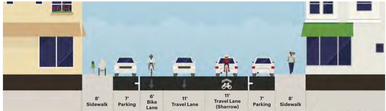
Near-term transformation (42' Curb-to-Curb)
