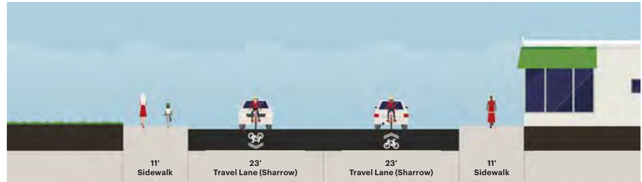
Existing condition (46' Curb-to-Curb). Note: Mostly "red curb" condition (no street parking allowed)
