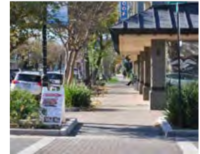
Figure 6.8 Wide pedestrian through-zones accommodate high levels of pedestrian activity in a downtown environment.
