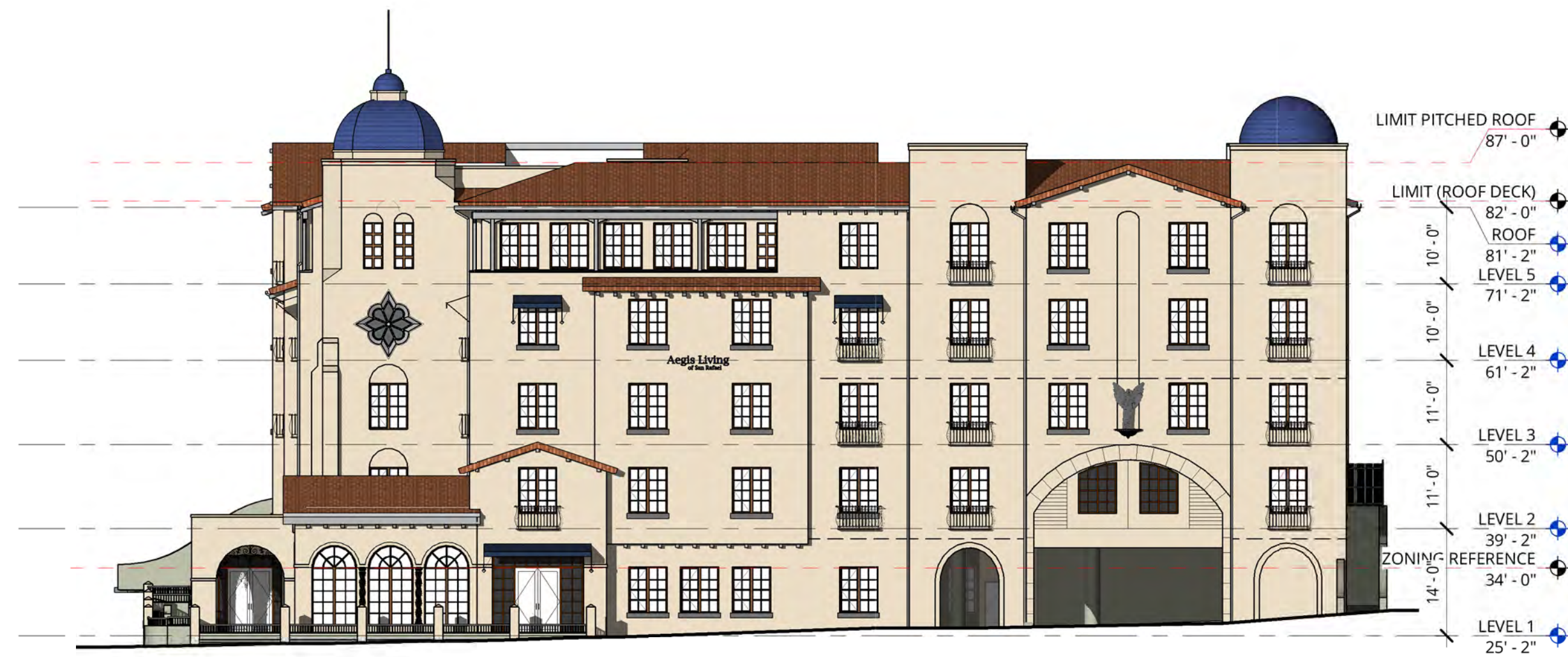
1 EAST ELEVATION - DRB IN MAY 2021 1/16"=1'-0"
