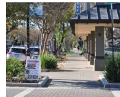
Figure 6.8 Wide pedestrian through-zones accommodate high levels of pedestrian activity in a downtown environment.
