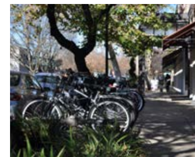
Figure 6.9 Furniture zones are ideal locations for streetscape elements such as bicycle racks and street trees.
