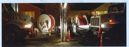
Two crews in hydroflusher trucks respond at night to prevent a sewer overflow during an intense storm event. These trucks contain powerful water jets with 2,000 pounds per square inch of pressure, root cutting tools, and powerful vacuums that are used to clean sewer lines and to clean up and prevent sewer spills.
