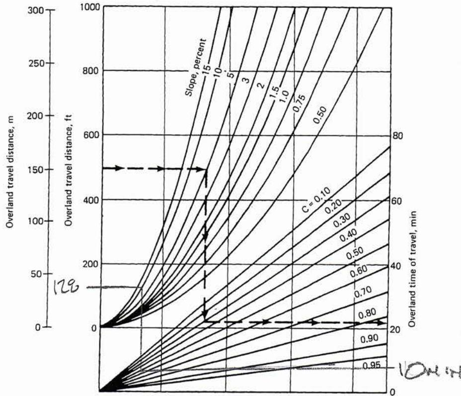
Fig. 4.5 A nomograph of overland flow time. (10) Enter left margin with slope length; move right to slope curve and down to C value; and find overland travel time on right margin.
