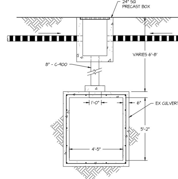
**STORMWATER CONNECTION TO EX-CULVERT**
