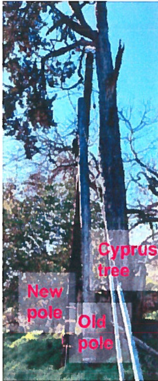
Figure 4. Soil subsidence and creep. The picture is taken where Ross Street Terrace, lot 45 (62 Woods Street), and the proposed driveway of lot #59 intersect. Note that the old utility pole and the cyprus tree are leaning in parallel to one another, while the new utility pole stands upright. Tree trunks of nearby oak trees are leaning in the same direction as the pole and the cyprus, demonstrating soil subsidence and creep. While only one location is shown here, indications of subsidence and creep can be seen in multiple locations on and surrounding the project site.
