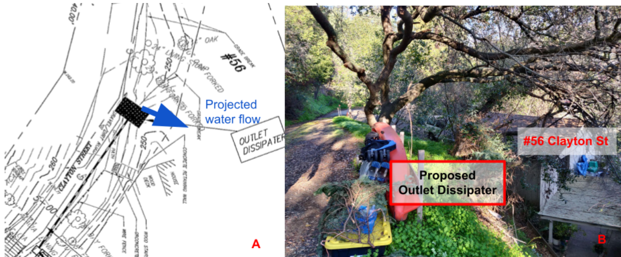
Figure 7. Proposed “outlet dissipater” location will flood #56 Clayton Street. A. The “outlet dissipater” as it appears on page 28 on the plans, with projected water flow overlaid. B. The existing terrain, showing the proposed “outlet dissipater” location, its proximity to #56 Clayton Street and the steep slope that the water will follow towards #56 Clayton Street residential structures.
