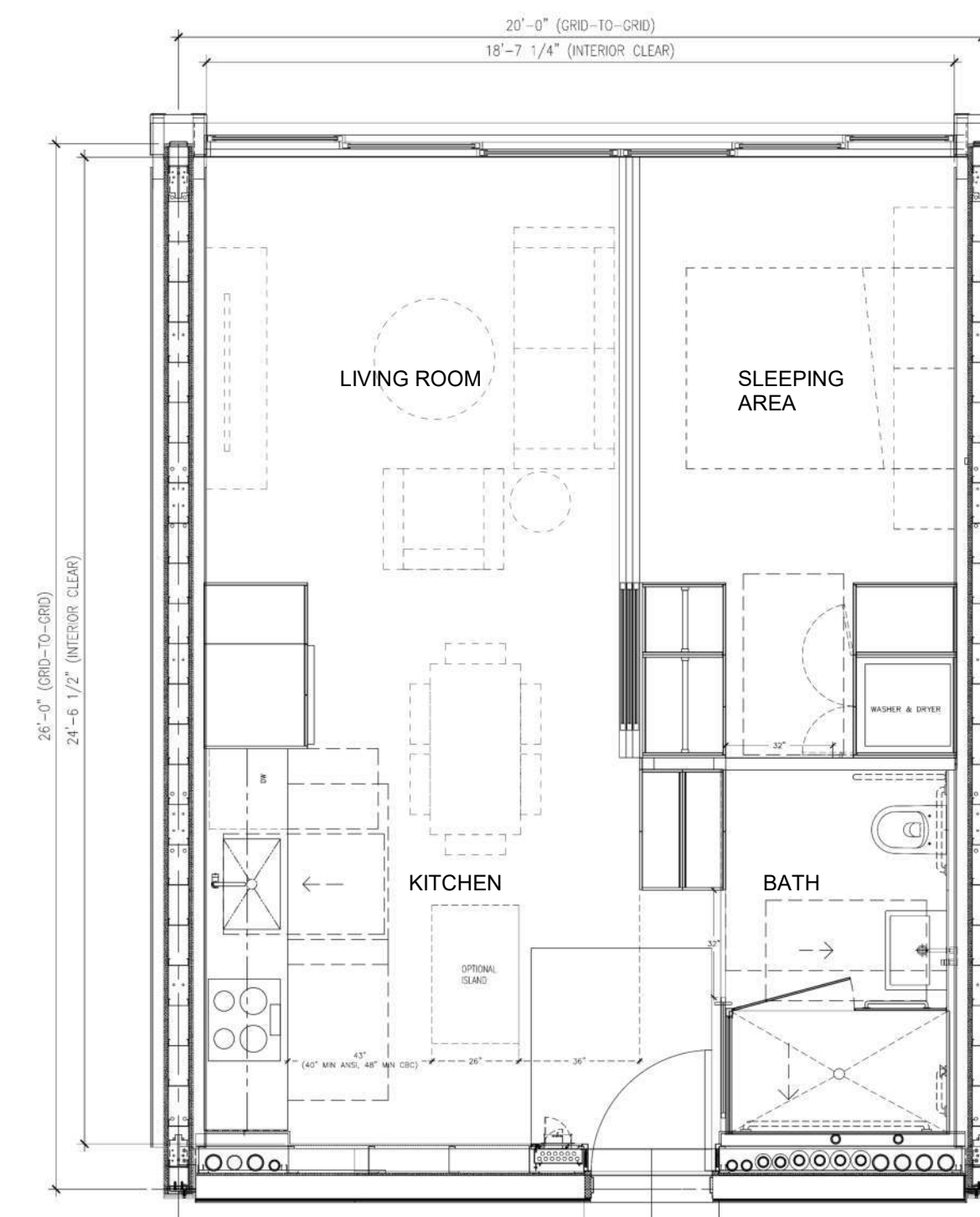
1 TYPICAL STUDIO UNIT A4.1 SCALE: 1/4"=1'-0"
