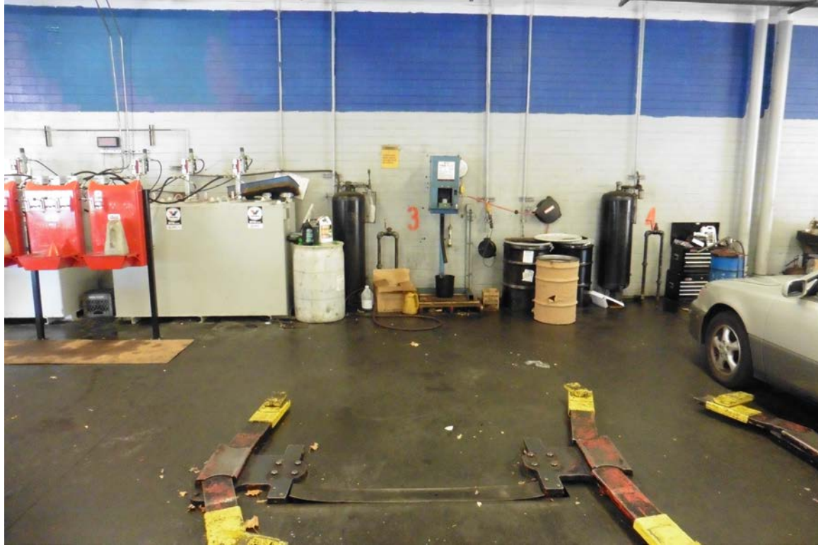
Photo 9: In-ground hydraulic lift and fresh oil AST storage at Sears Automotive Center.
