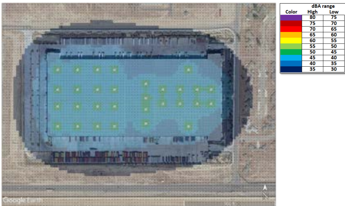
Figure 1: Aggregate operating sound emission from thirty (30) 8-ton (29 kW) air-cooled chillers (ACC) on a hypothetical warehouse rooftop.
