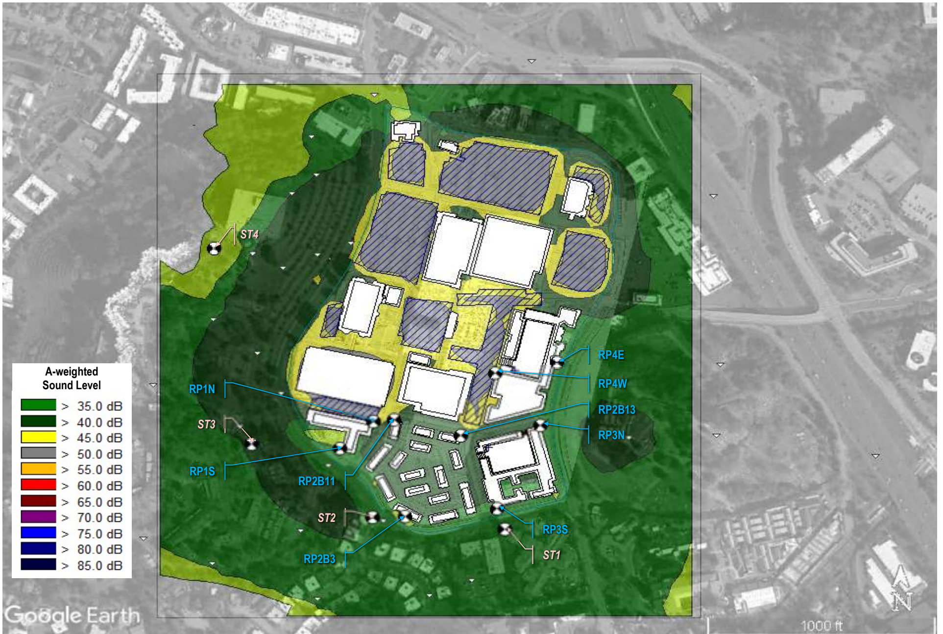
FIGURE 3A Predicted Stationary Source Operation Noise from Proposed Project - Master Plan - Daytime
