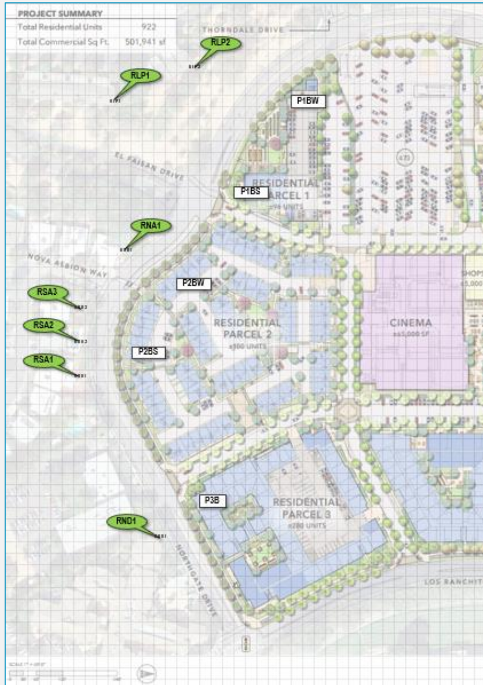
Exhibit E. Modeled Project Construction Activity Locations (white rectangles) and Noise-Sensitive Receptors (NSR, green oval callouts)
