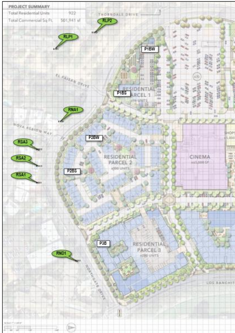
Figure B-1. Modeled Project Construction Activity Locations (white rectangles) and Noise-Sensitive Receptors (NSR, green oval callouts)
