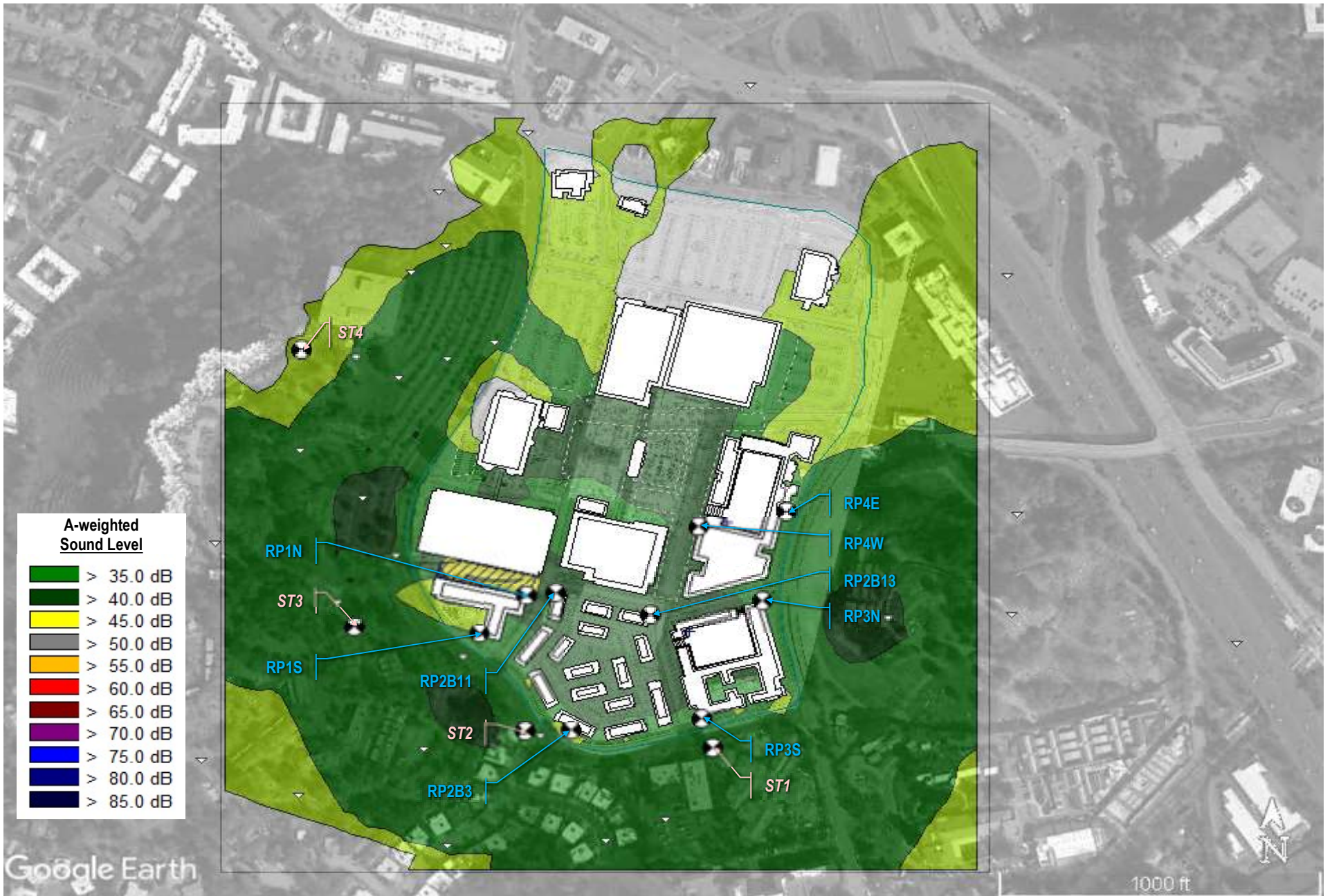
FIGURE 5B Predicted Stationary Source Operation Noise from Proposed Project - Master Plan - Nighttime with Cinema Occupied
