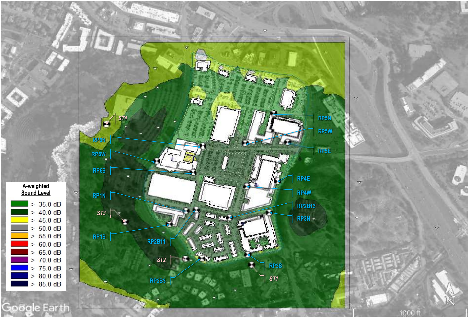
FIGURE 6B Predicted Stationary Source Operation Noise from Proposed Project - Vision Plan - Nighttime with Cinema Occupied
