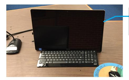
The power for the staff PC is located on the right side of the screen. Press this button to turn on the tablet PC.
