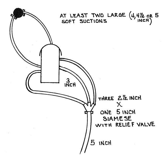
\* NOTE: If the engine pumping to the hose lay has a large diameter discharge, it may be used in lieu of the slamese with the three discharge lines.
