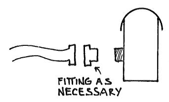
B. Connect the five inch hose to one portable hydrant. Adapt the five inch Storz outlet to 4 1/2 inch male thread. This creates the equivalent of a standard "steamer" hydrant at the scene that any engine company can connect to.
