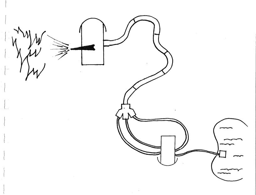
Dual Layout -- If the fire situation is extreme and the water supply <u>very</u> substantial, a dual layout could be considered.
