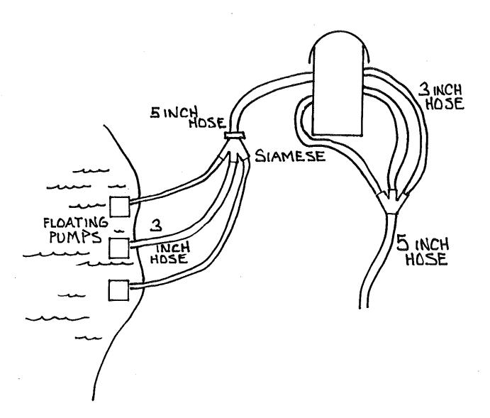
This evolution is capable of producing flows in excess of 1000 GPM.
