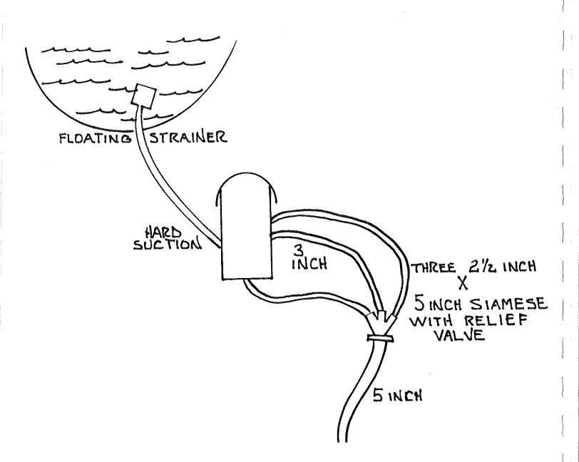
If a static source is not accessible or subject to depth changes, a Floto Pump supply can be established
