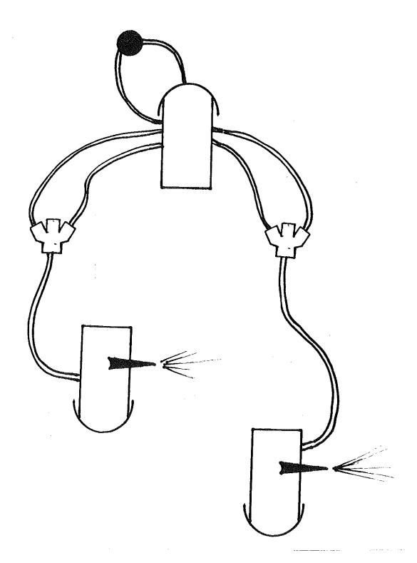
Relay -- In the case of a long layout or extreme elevation change with a high flow requirement, a relay may be considered.
