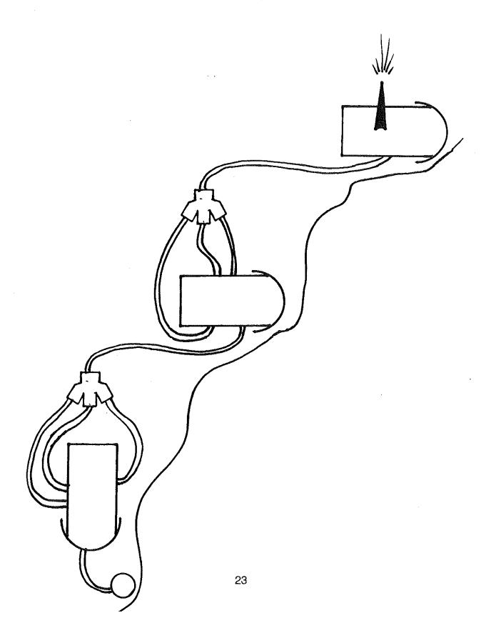
Portable Hydrants -- In the event that water sources are needed at multiple points along the hose layout, "portable hydrants" or manifolds can be installed. The manifolds have one 5 inch Storz inlet with one valved 5 inch Storz outlet and two 2 1/2 inch valved outlets.
